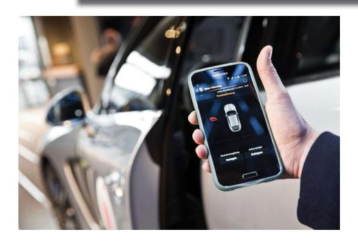
ave you had an experience where the vehicle notified the owner that it was being moved while it was in your repair facility? App-based connected services are available from many vehicle makers and may require special considerations before beginning repairs.
