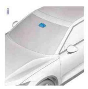
Calibration of the Forward Looking Camera is required after windshield replacement. Polestar systems are required to ensure correct functionality. Aftermarket services may find it quite difficult to properly re-calibrate stated systems.
