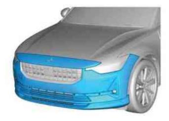
**Note!** In the event of damage in the form of holes or cracks within the marked areas, the component must be replaced. Do not repair the damage.
