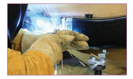
"Resistance spot welds should be placed adjacent to their original location(s) unless welding through multi-layer bonded joints."
