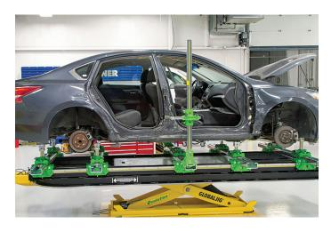
gaps could change. If the wrong measurements are used, it is also possible that weld-on panels will dent or buckle once the suspension is loaded or the engine is installed.
