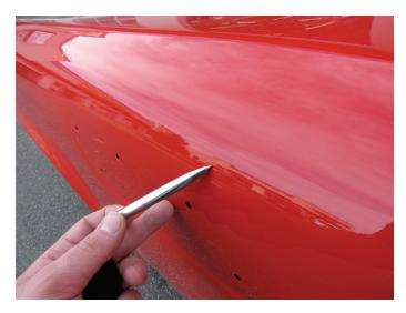
ometimes going back-to-basics can make the difference in a quality repair and a failed repair. Refinishing defects can take many forms and be influenced by the technician, environment, product selection, or equipment maintenance to name a few. Let's look at dirt nib inclusion during the refinishing processes.
