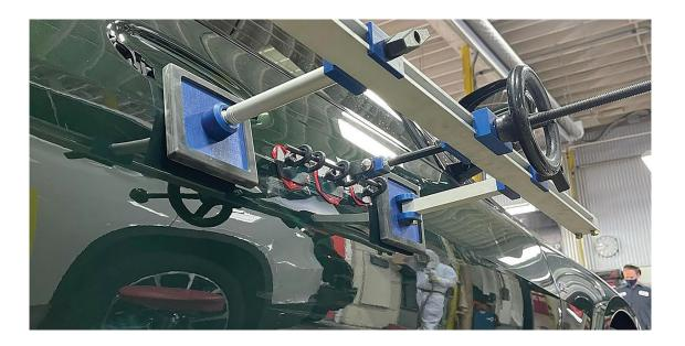
The next mistake that is commonly made occurs while positioning the replacement part. If repositioning of the part is needed, it is important to slide the part. Do not pick up the part and separate the adhesive. Lifting the panel introduces and traps air in the adhesive, weakening it at those points. Most panel bond manufacturers cover this in the technical data sheets (TDS) for the product.
