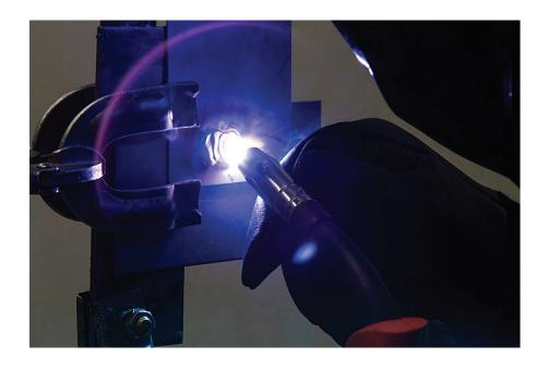
When it comes to MIG brazing, there are some common mistakes that are easily avoidable and can have a huge effect on the durability of the repair joint.
