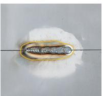
Generally, the melting temperature of the GMA welding electrode wire is higher than the evaporation temperature of zinc 910°C (1,670°F), causing the zinc to vaporize both in and around the weld zone. However, by reducing the welding temperature, less zinc will vaporize adjacent to the weld bead and the zinc disturbed by the process will "return."
