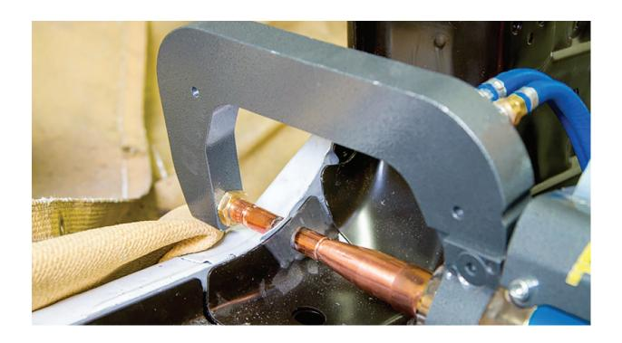
On today's vehicles, you are going to run into high-strength steel (HSS) and ultra-high-strength steel (UHSS) which will affect the attachment method that will be required when replacing body panels.
