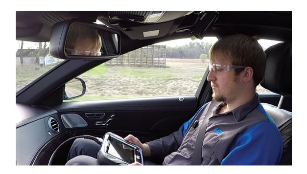
Many advanced driver assistance systems (ADAS) require a dynamic calibration procedure, or a static calibration followed by a dynamic calibration. A dynamic calibration requires the vehicle to be driven, often with two technicians and a scan tool. Though it can be easy to think of dynamic calibration as a test drive, they are not one in the same. Let's explore the difference between the two.
