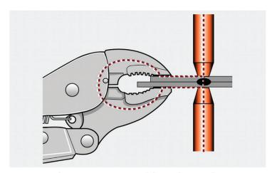
By using shunting, a spot weld can be made even though there is a coating on the mating surfaces.
