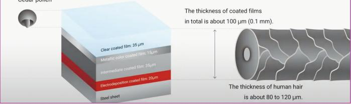
The average film build of E-Coat primer is 20 microns ( $\mu$ m = Micron) (that's around a fifth the thickness of a human hair!!)
