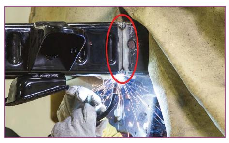
The other concern that becomes apparent with the indiscriminate removal of the E- Coating, is **thinning** of the base material from using inappropriate abrasive materials and tools that are too aggressive.
