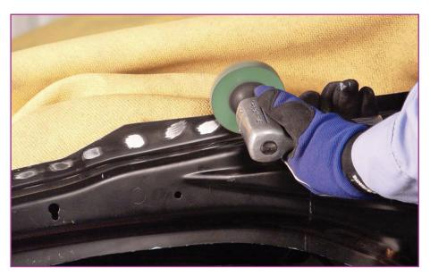
This includes sectioning joints to be welded -
