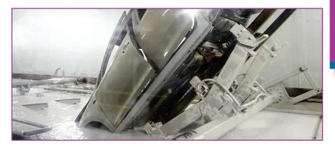
E-Coat or "Electrodeposition Coating" is a process used extensively by manufacturing industries around the world to provide a high level of corrosion protection on metal surfaces, with the added benefits of high productivity and cost efficiencies.
