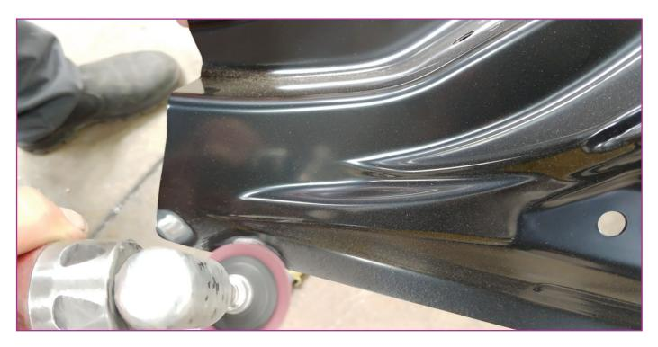
The opposite may be true for some OEMs -Honda have recently updated their recommendations when working with 1500 MPa tensile strength Hot Stamped Steels (targeting the "door ring") – the protective aluminium sheet metal coating must be carefully removed (along with E-Coat), prior to welding...
