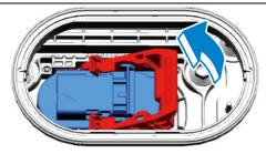
Press the area indicated by arrow shown in the figure, release the tabs, and then raise the lever until it is perpendicular.
