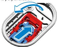
➤ Hold the lever and pull the service plug straight up.
