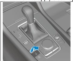
Pull the electric parking brake (EPB) switch up.
