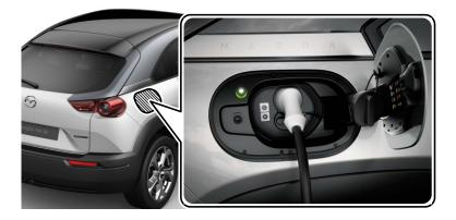
The charge port has a lock function to prevent the charge connector from being unplugged due to vibration or mischievous behavior during charging.
