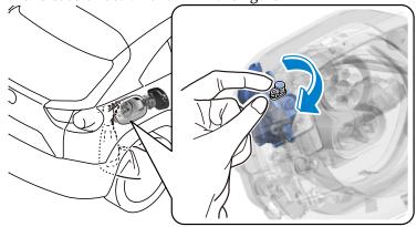
3) Remove the charge connector with the charge connector lock manual release lever pulled.
