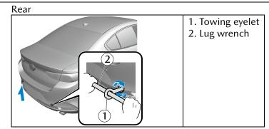
4) Attach a rope to the eyelet.
