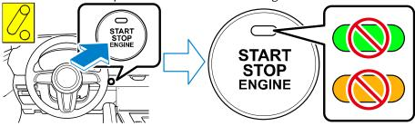
2) Keep the key 5 m {16 ft 5 in} or farther away from the vehicle so that the system does not restart.
