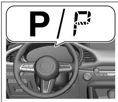
When the transmission is in the P position with the power switch switched ON, the selector lever position indication is [P].
