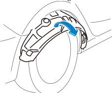
2) Insert a hand from inside the tire housing and pull the charge connector lock manual release lever in the release direction shown in the figure.
