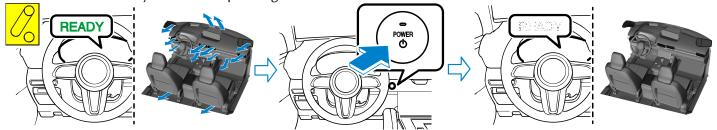
2) Keep the key 5 m {16 ft 5 in} or farther away from the vehicle so that the system does not restart.
