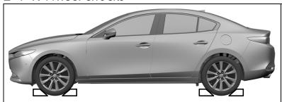
Use the wheel chocks at the positions shown in the rescue sheets for each vehicle model so that the vehicle is secured firmly.
