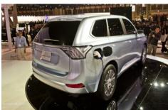
The Mitsubishi Outlander PHEV is a 300 volt electric vehicle with both series and parallel hybrid functionality. It incorporates a 2 litre internal combustion engine which can drive an on-board generator and or the front wheels directly.
