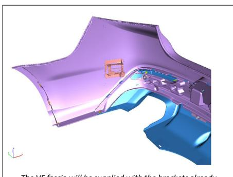
The VF fascia will be supplied with the brackets already welded on
