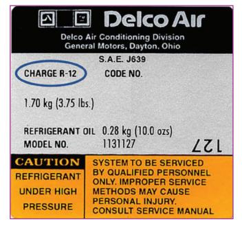
In the 1990's, law changes put a ban on CFC – based fluids as these were seen to have an adverse affect on the ozone layer. For the most part, vehicle-makers had already developed, and were using alternative refrigerants. The chosen fluid was **R134A** – a type of **Hydro Fluoro Carbon (HFC)** which has a zero rating for ozone depletion.
