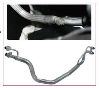
An inline heat exchanger (IHX) has concentric inner and outer chambers. Liquid refrigerant from the condenser flows through the main inside chamber, and the outside chamber surrounds it with vapor from the evaporator.
