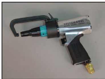
Figure 2 - A pneumatic C-clamp-style drill applies adequate pressure to the cutting bit.
