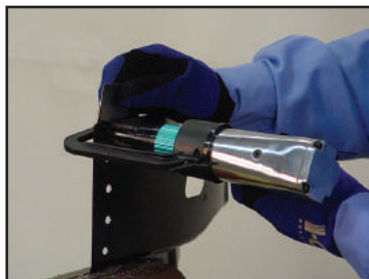
Figure 3 - A C-clamp-style spot weld drill is also effective for making plug weld holes in a UHSS part.
