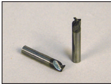
Figure 1 - A triple-fluted tungsten carbide bit effectively removes spot welds from UHSS alloyed with boron.
