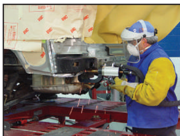
Figure 6 - This spot welder pulses to preheat the metal before making the weld.
