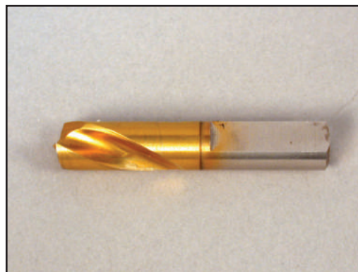
Figure 3—A titanium drill bit such as this worked on boron steel.
