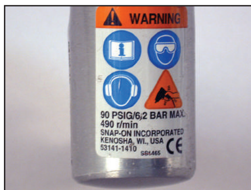
Figure 4—This special 490 rpm air drill motor was essential for drilling out spot welds from boron steel.
