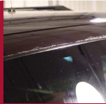
Figure 1 - Corrosion along the windshield pinchweld can cause leaks into the vehicle interior.
