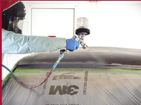
Figure 5 - Anti-corrosion primer must be applied to the pinchweld to reinstall corrosion protection over the bare steel.
