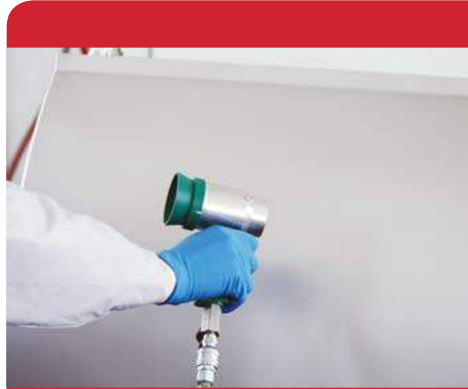
Figure 2 - Hand-held air multipliers are one example of equipment that can be used to provide increased air movement to aid drying efficiency of waterborne materials.
