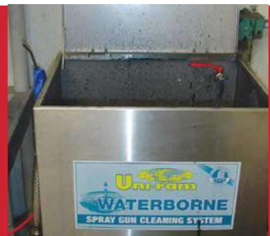
Figure 1 - Cleaning a spray gun used to apply waterborne materials may require specific solutions (left) and equipment (right).
