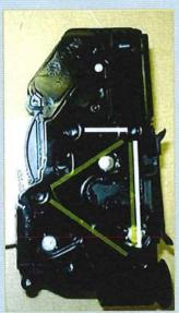
Rear door latch with four mounting points - "triangular pattern" & "L-shaped pattern"
