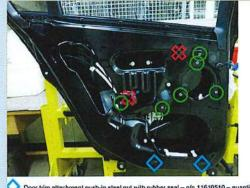
Door trim attachment push-in steel nut with rubber seal - p/n 11610510 - quantity 2
