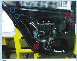
Seal hole with adhesive Mylar patch - 92196496 - quantity 3 per door
