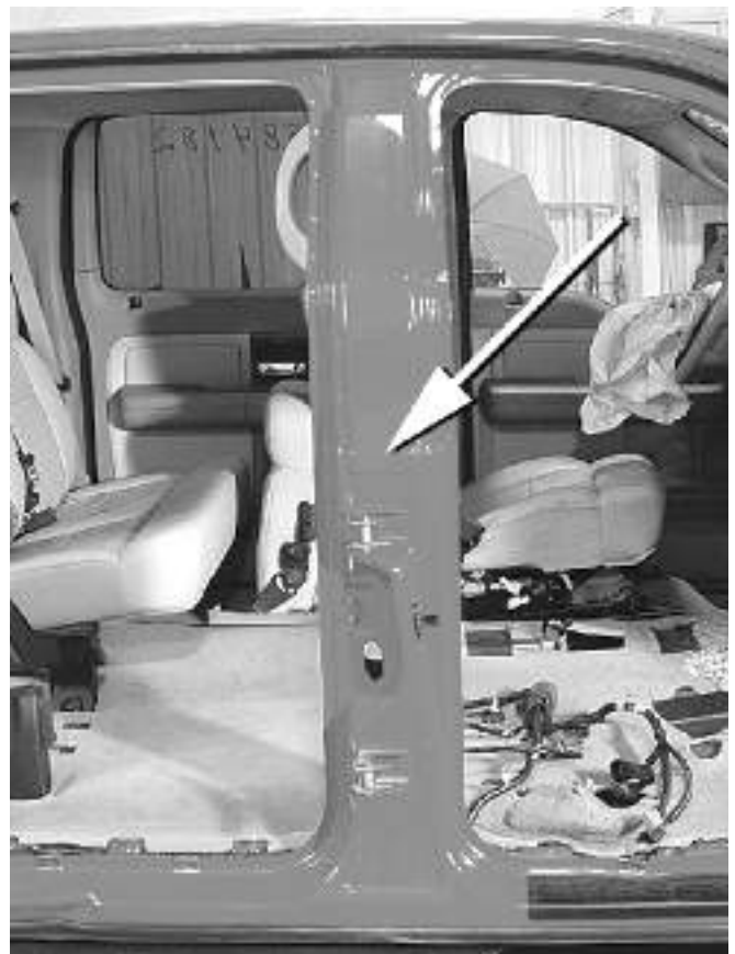
Figure 9 - The center pillar on this Ford F-150 uses a tailor-welded blank.
