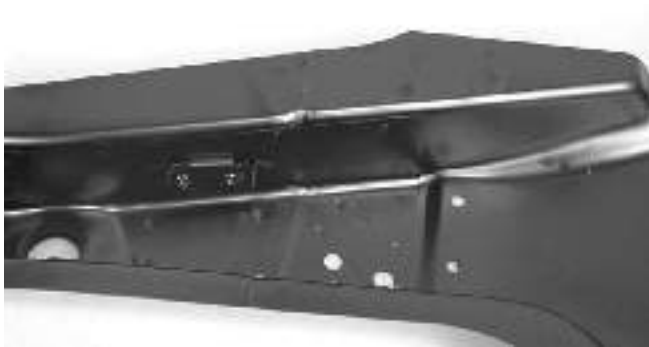
Figure 7 - High-strength and extra-high-strength steels are joined at the lower portion of this inner B-pillar.
