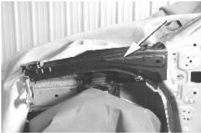
Figure 3 - The upper front rail, or side member, on the Volvo S40 is a two-part tailor-welded blank.
