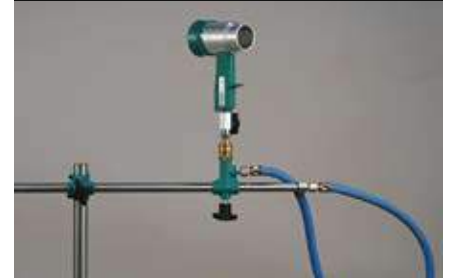
Figure 7 - This is an example of a hand-held air multiplier mounted on an adjustable stand.
