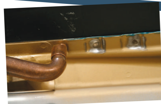
Figure 1 - When attaching a third panel to an originally weld-bonded panel, the recommendation from at least two vehicle makers is to use no adhesive and the original weld locations.
