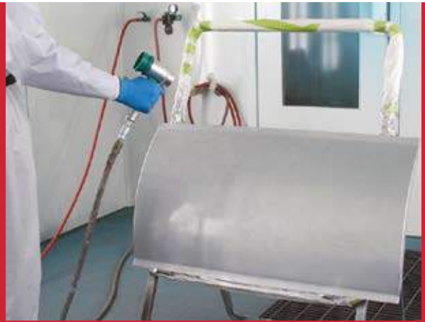
Figure 8 - Air multipliers improve flash time of waterborne basecoats.
