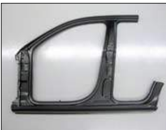
Figure 3 - This is the service part that the outer rocker panel must be cut from, no matter which procedure is used.
