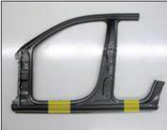
Figure 2 - The outer rocker panel may be sectioned in either of these two shaded areas.
