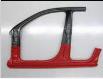
Figure 1 - Before earlier in March, the only procedure in the service information for replacing the outer rocker panel was the entire outer rocker panel.
