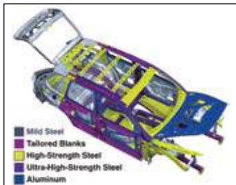
Figure 7 - Advanced high-strength steel is used throughout the Cayenne body.
