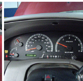
Figure 4-The engine is started and the instrument panel is inspected for any diagnostic trouble codes.
