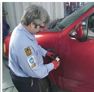
Figure 3-A gap gauge as well as a visual inspection ensures that the body panels are in alignment.
