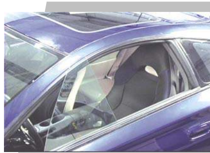
Figure 1 - Because of reflections, glass will pick up colors from items around it and its true tint color may be difficult to determine.
