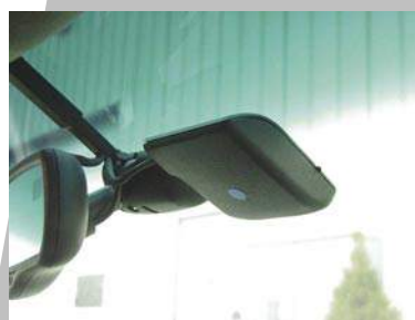
Figure 2 - This moisture sensor is highly visible.
