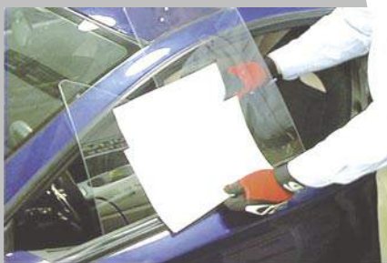
Figure 5 - When compared to clear glass it is readily apparent that this glass is tinted, but its true color is difficult to determine.
