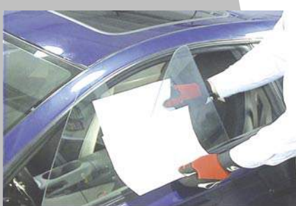
Figure 4 - With the white paper behind them, comparing the colors to each other makes it quite apparent which glass is blue and which is green.
