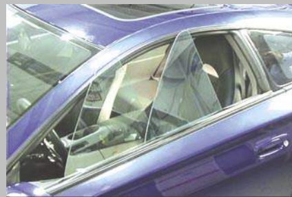
Figure 3 - This blue and green glass placed side by side shows the subtle difference between the two tints and illustrates the difficulty of determining the correct color.
