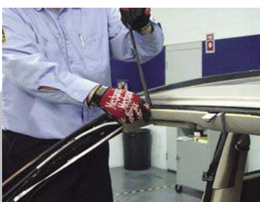
Figure 1 - The last step with a full cutout is trimming the urethane adhesive to a final 1–2 millimetre height.
