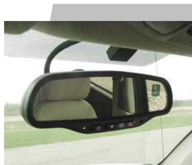
Figure 1 - This rearview mirror includes an automatic dimming feature, a compass, an outside temperature reading and GPS.
