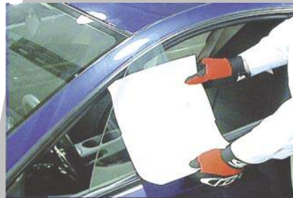
Figure 2 - Using the white paper test makes the tint color of the glass jump out at you, but it can still be difficult to tell whether the glass is blue or green.
