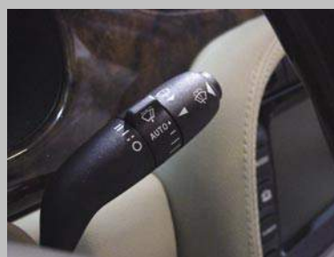
Figure 3 - This moisture-sensing system is operated using a separate switch on the steering column.
