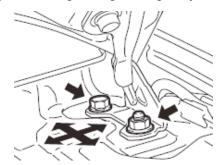
Front door hinge mounting bolts tightening torque: 27  $\pm$  5 N•m
