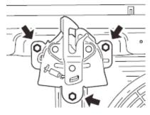
Hood hinge mounting bolt tightening torque:  $22 \pm 4$  N•m Hood hinge mounting nut tightening torque:  $12 \pm 2$  N•m
