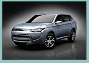
The Mitsubishi Outlander PHEV is a 300 Volt Electric vehicle with both series and parallel hybrid functionality. It incorporates a 2litre internal combustion engine which can drive an on-board generator and or the front wheels directly.
