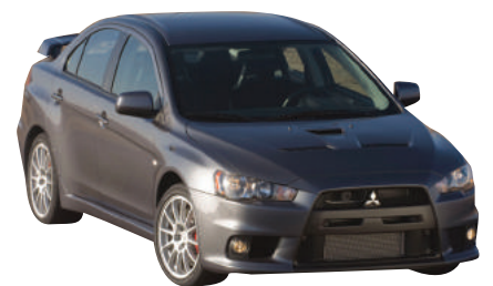
This 2008 Mitsubishi Lancer Evolution has a rivet-bonded aluminium roof panel.
