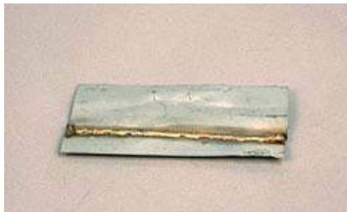
Figure 4—The bead of a MIG-brazed weld should not lay flat on the joint.
