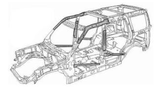
No attempt should be made to straighten Ultra High Strength steel, due to its brittleness.
