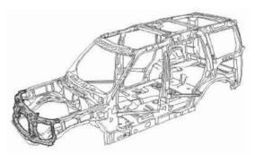
No attempt should be made to weld or straighten the hood latch panel and it should be replaced in the event of an accident. If the corrosive coating is damaged it must be repaired using 'Land Rover Low Temperature Anti-Corrosion Coating', service part no VEP 501 840 PMA
