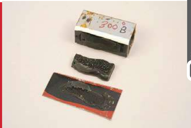
Figure 3 - The sample shows substantial degradation of the urethane adhesive.
