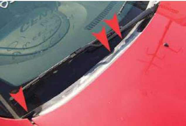
Figure 2 - The plastic trim panel at the bottom of the windshield started to warp from excessive heat, caused by a vehicle fire.
