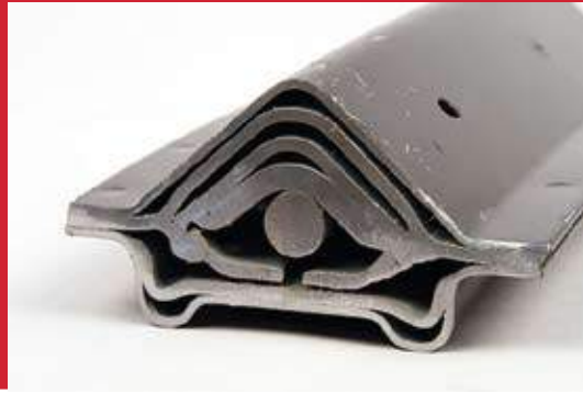
Figure 1 - A cutaway of a B-pillar from a 2000 Subaru Legacy Outback wagon shows multiple reinforcements.
