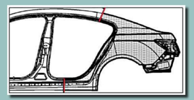
Looking at the B Pillar outer panel replacement; this is another standard GM repair method for models that have ultra high strength steel (UHSS) reinforcements, this requires cutting into the cant rail to allow assess for fitting the full reinforcement. There is also a method for fitting the B Pillar reinforcements. Fig. 6 shows the B pillar outer panel removed.
