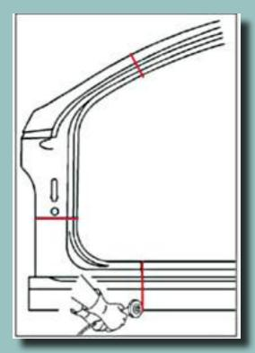
The sill (rocker) and B pillar outer panels plus the inner reinforcements are almost a reproduction of the VE Commodore method but the Malibu does have different measurements so these should be followed. The full outer sill panel can be fitted (see Fig. 4) but remember the other joint locations for the A and B Pillar or rear quarter can also be considered.
