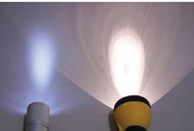
Figure 4 - Different colored light may help show corrosion.
