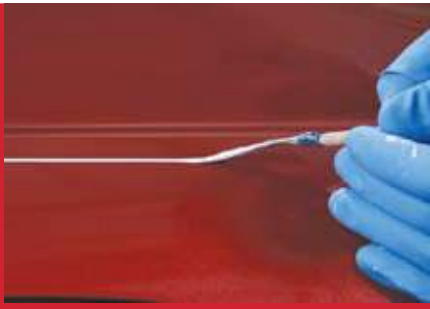
Figure 6 - Pinstriping brushes are designed to hold an adequate amount of paint so that long lines can be created without having to constantly dip the brush back into the paint.
