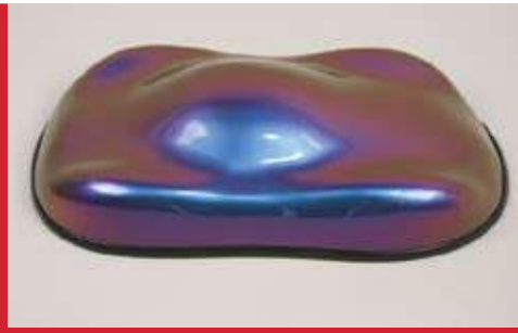
Figure 4 - Colour-shifting topcoats give the finish a different colour appearance depending on the angle the finish is being viewed.
