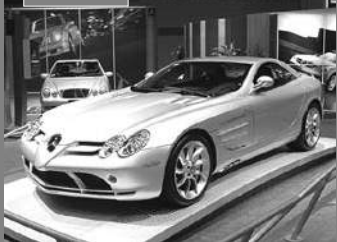
The 2003 Mercedes-Benz SLR McLaren has the complete front structure made from CFRC.
