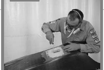
Plastic repair material is used to repair the damage on this Corvette Z06 fender.
