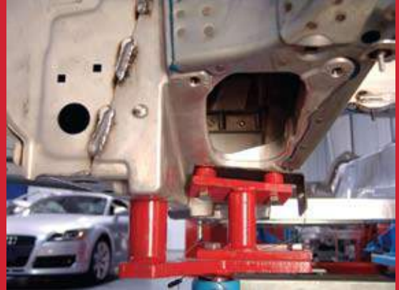
Figure 5 - The torque boxes on the Audi TT are made from cast aluminium.
