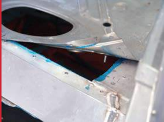
Figure 4 - The adhesive provides protection against galvanic corrosion where steel and aluminium are joined.
