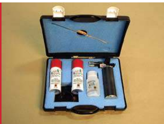
Figure 2—The Pyrosil® (flame) kit is used to prep flanges for adhesive application.
