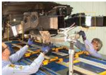
Figure 10 - The Corvette Z06 may be sectioned in five locations on each side.
