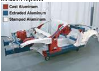
Figure 5 - The Jaguar XK uses an advanced monocoque construction.
