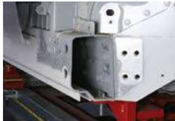
Figure 6 - Open extrusions are used for the Jaguar XK inner and outer rocker panels.
