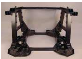
Figure 4 - A complete Audi R8 rear structural assembly is available for collision repairs.
