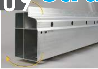
Figure 1 - Multi-celled extrusions have high resistance to twisting.
