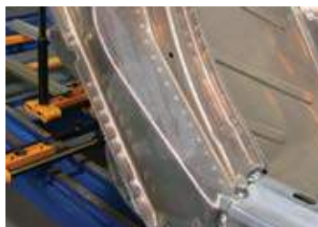
Figure 9 - The B-pillars are stamped aluminium joined with self-piercing rivets.
