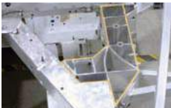
Figure 3 - Extrusions are used in place of castings for connecting the front rails to the center structure.
