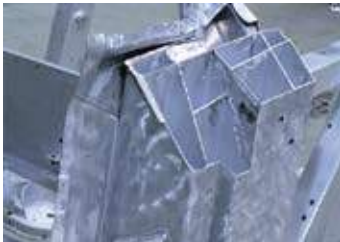
Figure 2 - The extruded inner B-pillar on the Audi R8 has eight cells.
