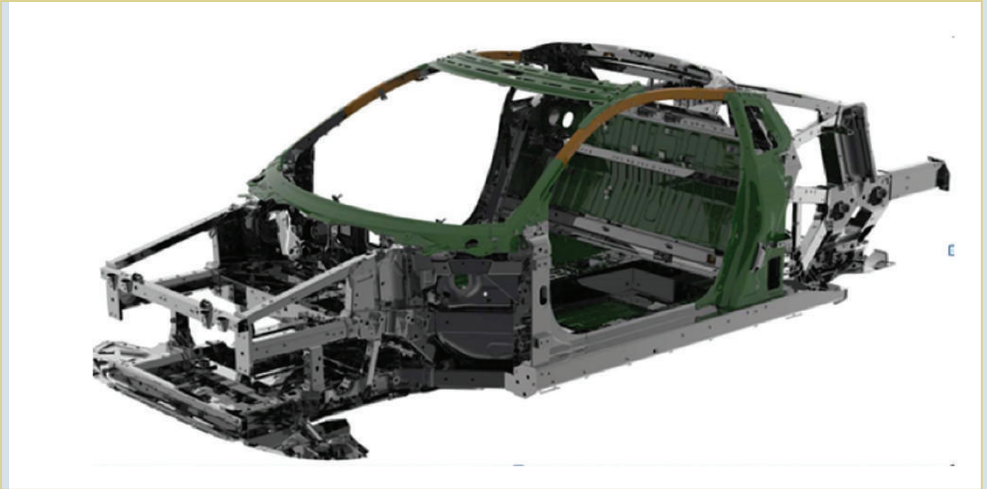
HONDA NSX - for the most part, an aluminium structure, with some HSS (590Mpa ) shown in Green and UHSS (1500Mpa ) shown in Brown.
